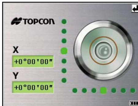
Rotate the leveling screws while observing the display.
