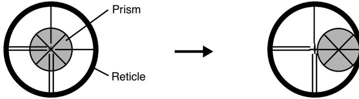
**7** Turn the horizontal jog clockwise slowly, and move the collimating point to the prism center gradually until at the position buzzer starts. Confirm the level of the signal (light quantity level) in display to adjust at the level of one to two as shown in below by turning the horizontal jog.
