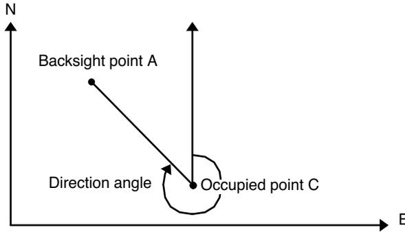
Example: Occupied point C : N coordinate 5.321m, E coordinate 8.345m
