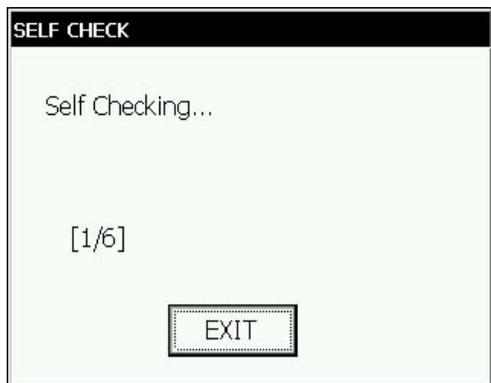
The instrument will turn automatically and the tilt sensor offset value will be measured and memorized.
