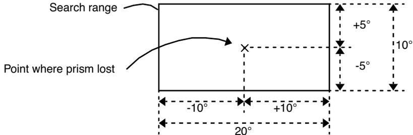
Setting Search range requires consideration. The items to think about: optical path interrupted by other objects; collimated point from IS series to prism is shifted after Turning and Searching Command; possible other prisms, targets, or other objects to interfere with tracking the desired prism; and many other examples all play a role in determining the search range.
