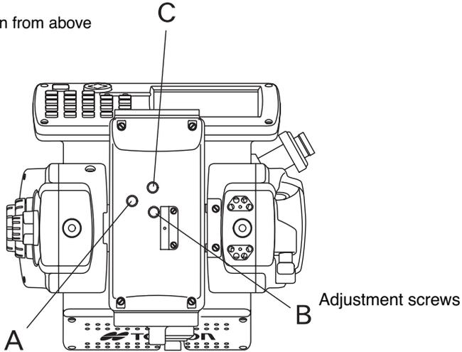
When screws A, B and C are turned clockwise (the direction for tightening them), the laser pointer, as seen on the target from the standpoint of the IS, will move in the direction shown in the drawing.
