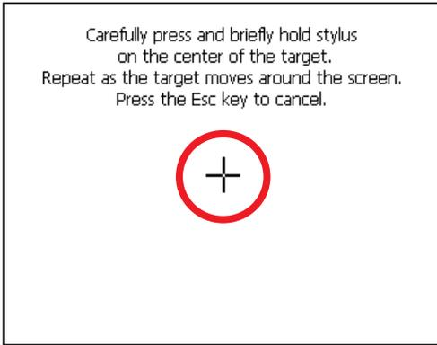
4 Using the stylus pen, press the center of the targets on the screen.
