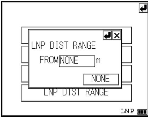
4 Input the distance range by pressing the numeric key. \*1)
