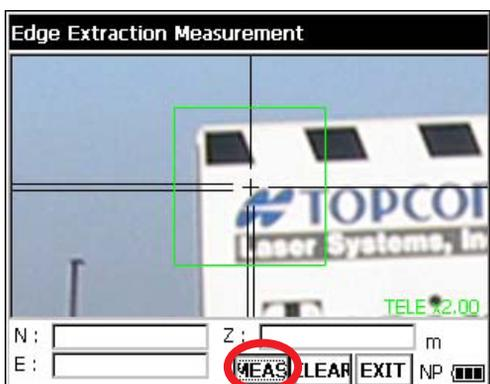
3 Switch to the telescopic mode and press the [MEAS] key.
