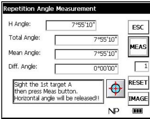
The total of angle and the mean of angle are shown.
