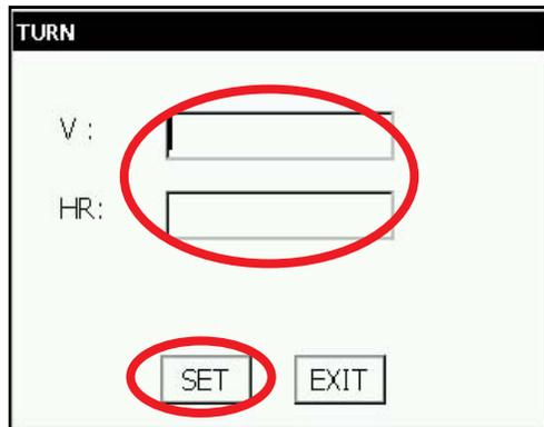
**1** At angle measuring mode (Page 3), press the [TURN] key.
