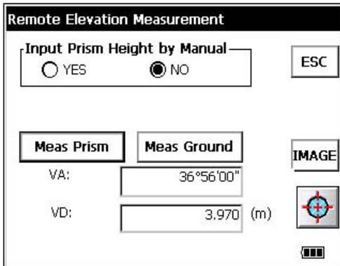
9 Collimate target K. Vertical angle(VA) and Vertical distance(VD) will be shown.
