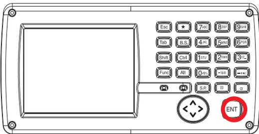
5 After pressing all targets (5 points), press the [ENT] key, or tap the display.
