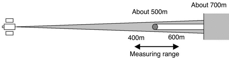
To set measurement distance range, see Section 4.3.3“Setting Measurement distance range of Non-prism long mode” .
