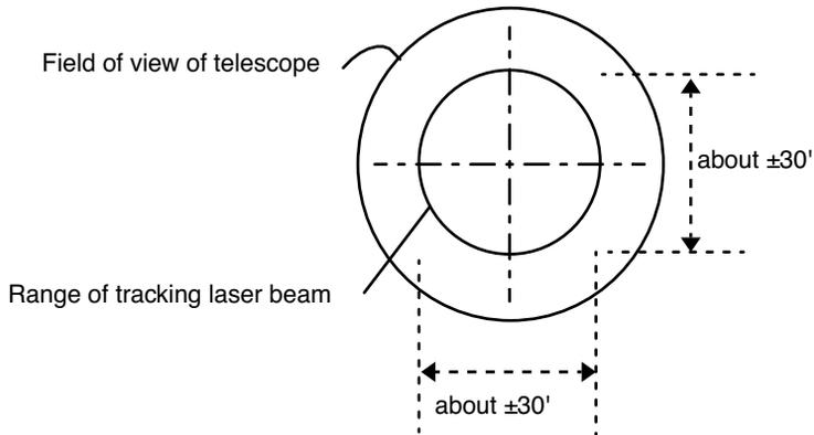
The range of the laser beam for auto-tracking in a short distance is almost the same as a telescopic field of view. Therefore, quick starting of auto-tracking and auto-collimating are possible if the prism is contained in the telescopic field of view.
