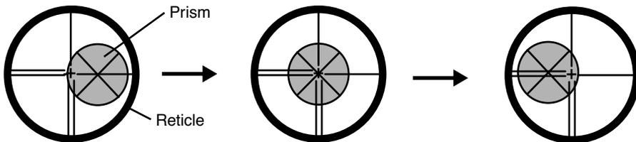
**10** Move the collimating point to the center of prism gradually until buzzer sound starts. Turning the horizontal jog to be one to two level of SIG value to adjust the collimating point same as step 7 procedure.
